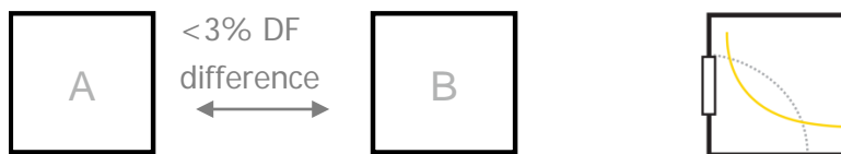
Figure 5. The difference between two adjacent rooms should not exceed a daylight factor of 3%. Rooms with windows at only one side should be wide but not deep.
